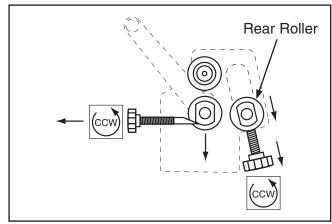
Figure 13. Slip roll preparation.
